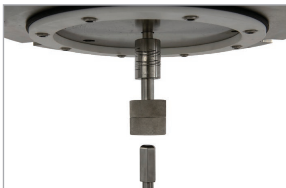
View of Stir Shaft and Upper Coupling
