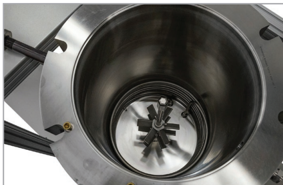
View of Stirrer and Spiral Cooling Coil
